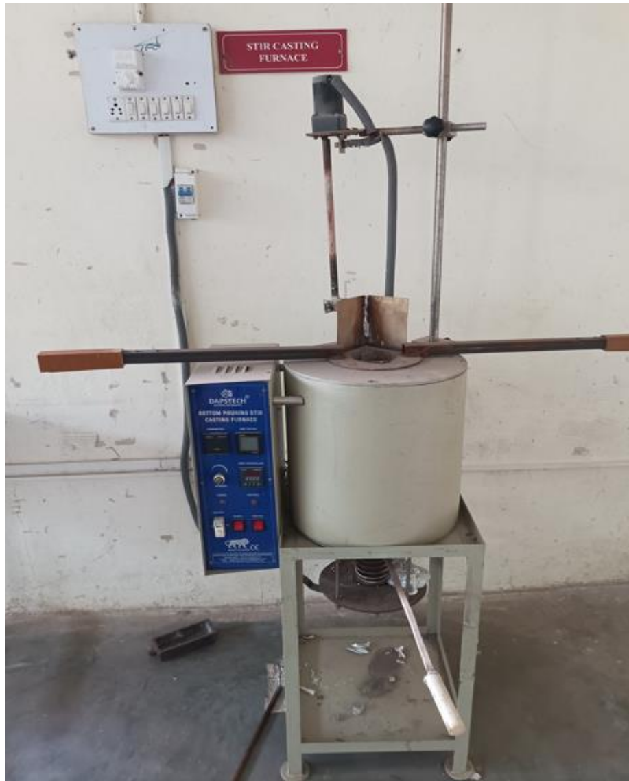
Fig: Induction Furnace with stirring arrangement.
